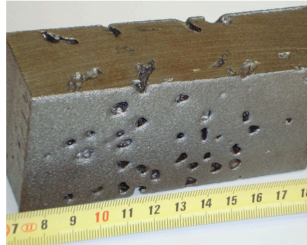
Gasporosität in GS-20Mn5 - Gussstahl at wikipedia - CC-BY-SA 3.0
