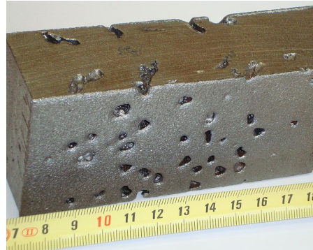
Gasporosität in GS-20Mn5 - Gussstahl at wikipedia - CC-BY-SA 3.0
